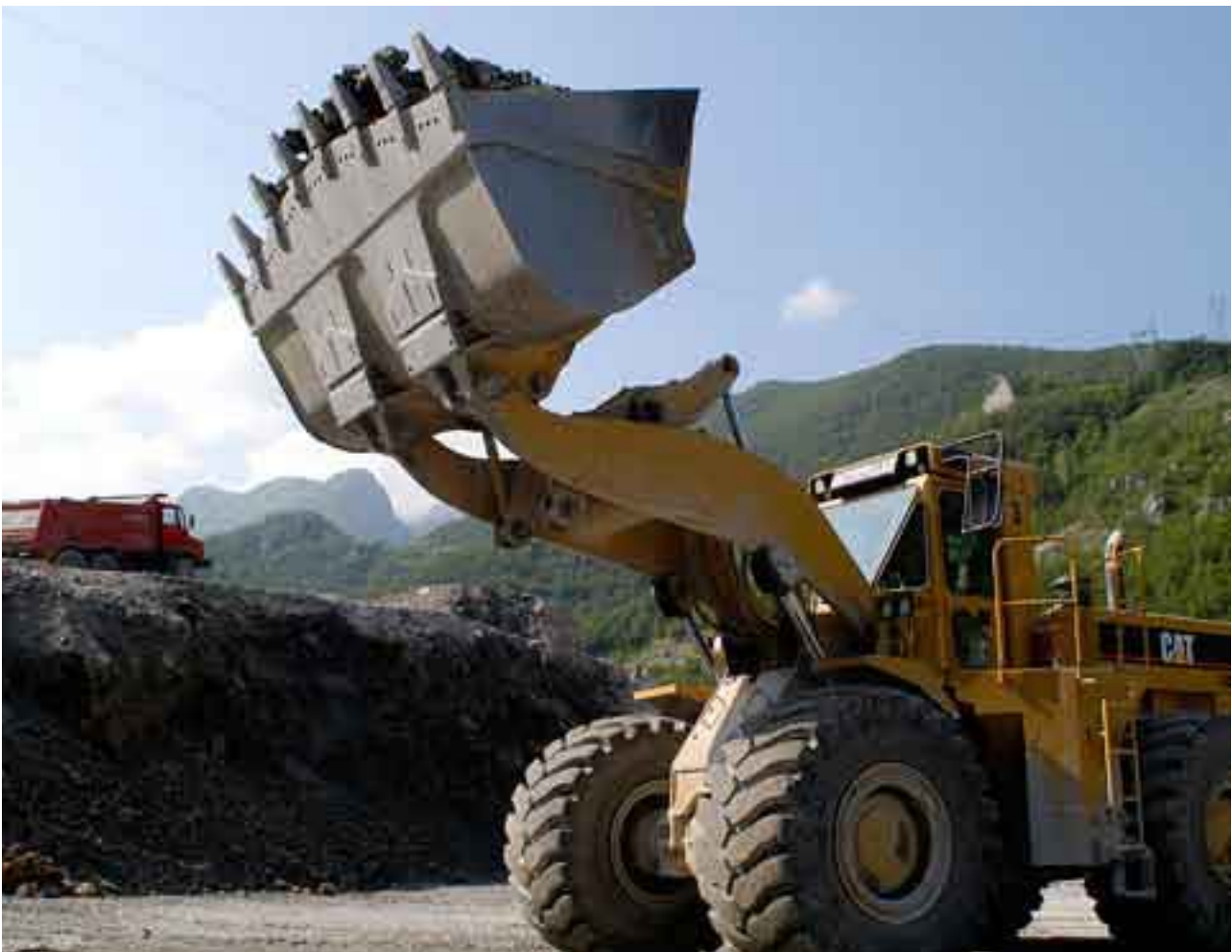
Robilante, Italia: pala gommata al lavoro in cava calcare Robilante, Italy: wheel loader working in the limestone quarry
