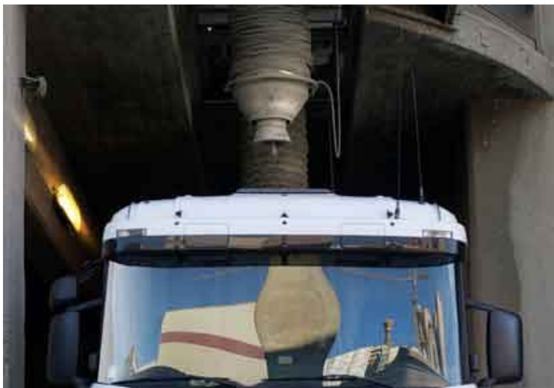
Cisterna carico cemento sfuso Silotruck loading bulk cement
